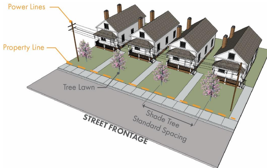
Figure 6-2: Street Trees Placed in Front Yard (outside of ROW) when Overhead Power Lines are Present
